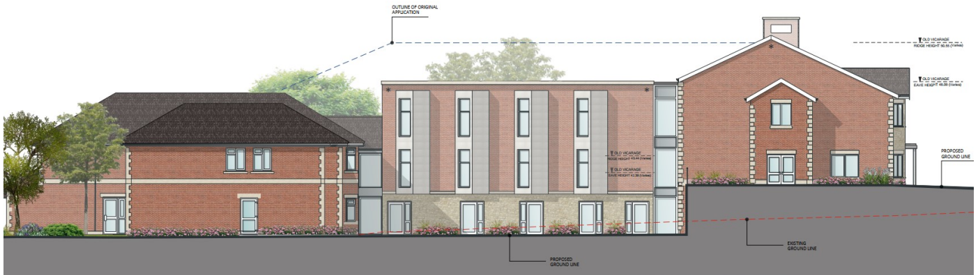
Revised Proposed 'Elevation A' – The blue line shows the height of the previously proposed pitched roof. Dotted line shows the existing ground level of the boundary with No 50b
